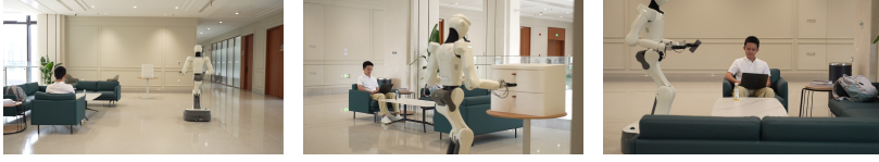
(a). The robot executes a long-horizon sequence of navigation and manipulation, composed at run time, to retrieve and deliver a power bank.
