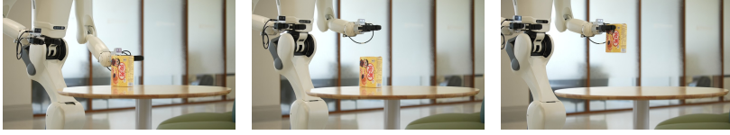
(c). The robot uses the evaluator's failure reason to reposition relative to the object and complete the grasp after the initial attempt fails.
